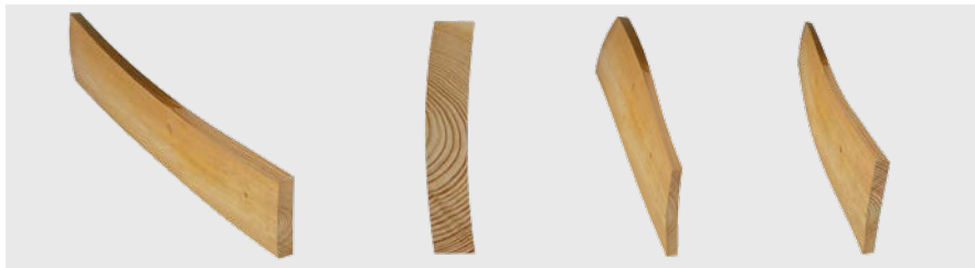
Blocks with longitudinal/latitudinal deformation, cupped or warped
